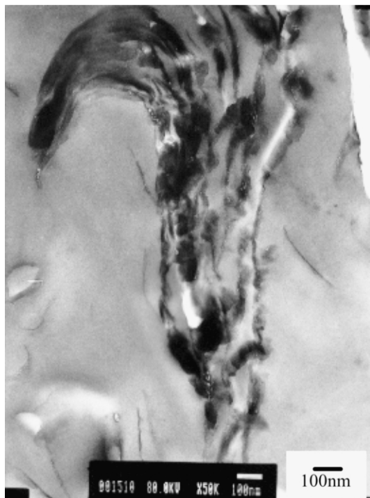
Fig. 1. TEM of BisAPAF-PMDA polyimide/3 wt% clay nanocomposite prepared from BisAPAF-PMDA polyamic acid n -butyl ester.
